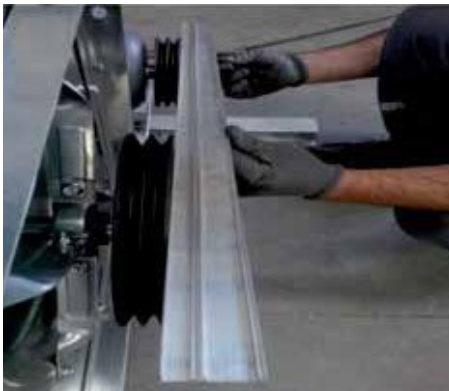
Image 7. Alignment Check of Pulleys-2
