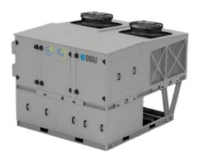
**ECRH - ECO:** The ECO series is equipped with economizer dampers at the fresh air intake, return air, and exhaust outlet. The unit operates with a 30% fresh air ratio, which can increase up to 100% with natural cooling depending on external air conditions. The economizer dampers are controlled by precise sensors on the fresh air and return air streams.
