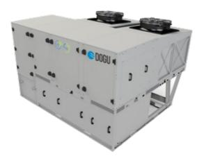
ECRH - ENERGY: The ENERGY series units are designed with economizer dampers and a rotary heat recovery system, making them ideal for areas with high fresh air requirements. Through a highefficiency, low-pressure-drop heat exchanger, both sensible and latent heat transfer occurs between the exhaust air and fresh air, ensuring efficient energy recovery.
