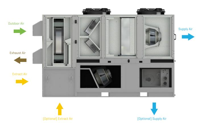
In the ECRH ENERGY model with heat recovery and economizer dampers, heat recovery and thermodynamic heat recovery are carried out by the return fan. A portion of the exhaust air is mixed with fresh air according to the mixing ratio and then passes through the rotary-type heat recovery unit.
