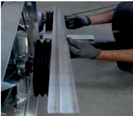
Image 7. Alignment Check of Pulleys-2
